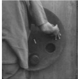
3. Slide the first Cell-Cast® disk over the \*threaded rod. **Note:** Use only 1 threaded rod for equal distribution. More than one rod could take disks out of shape.
